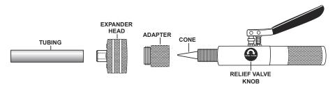
1) Use soft copper tube or heat (anneal) the section of hard copper tubing to be expanded.
