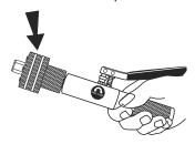
6) Place the tubing onto the expander head. Make sure that the expander head travels into the tube FRFFLY.
