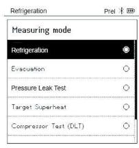
3 Press [▲] / [▼] to select Pressure Leak Test and press [Menu/Enter] to confirm.
